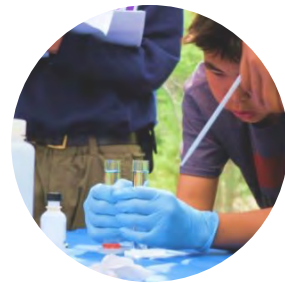
Manual measurement of turbidity with Morgan
